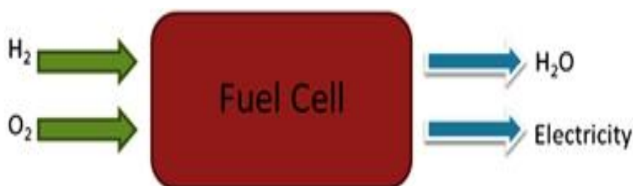
General concept of a H 2 -O 2 fuel cell
